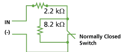
Figure 7: Normally Closed Supervised Input with Double Resistors
